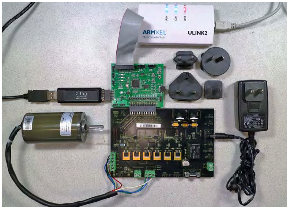
Figure 6. The MultiMotor Development Kit with Z32F128 MCU Module and Keil ULINK2 Debugger
