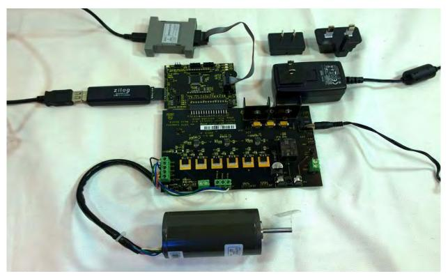
Figure 4. The MultiMotor Development Kit with the Z51F3220 MCU Module and OCD Cable
