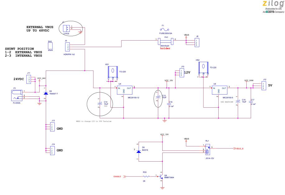
Figure 9. MultiMotor Development Board, #2 of 2
