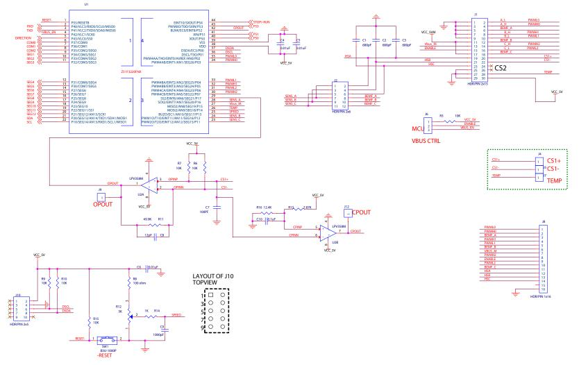
Figure 6. Z8051 MultiMotor MCU Module, # 1 of 2
