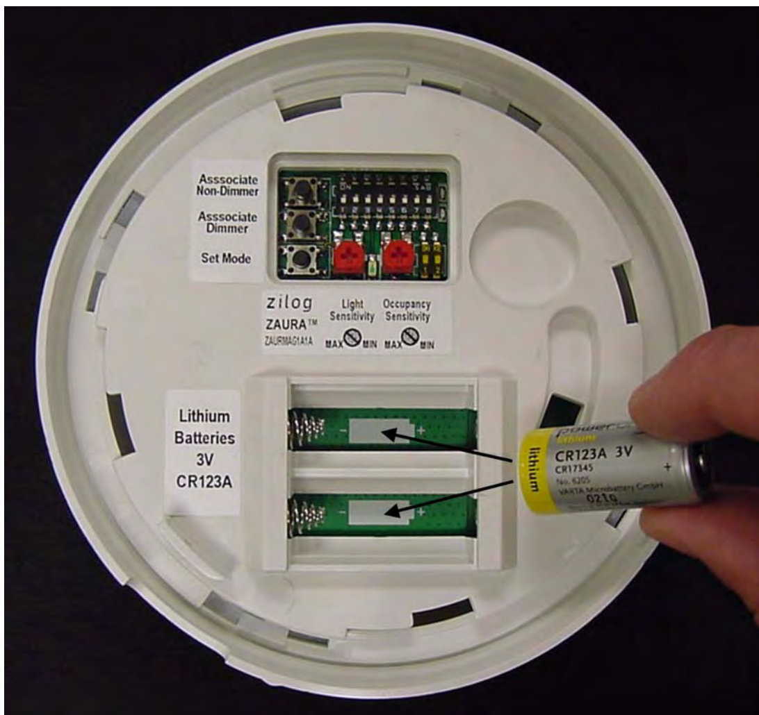
Figure 20. Master Unit Battery Installation
